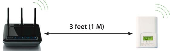
**Minimum 3 feet (1 M) between Wi-Fi equipment and Vykon wireless devices**
